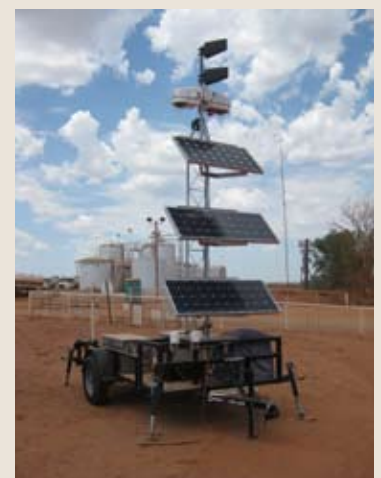
A typical remote installation deployed by one of the top three leading producers of natural gas at over 500 sites. One IR illuminator and two VideolQ HD cameras are powered completely by solar and utilize a wireless 3G connection.
